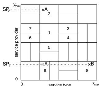
Figure 2: A two-dimensional CAN for discovering services and service providers
