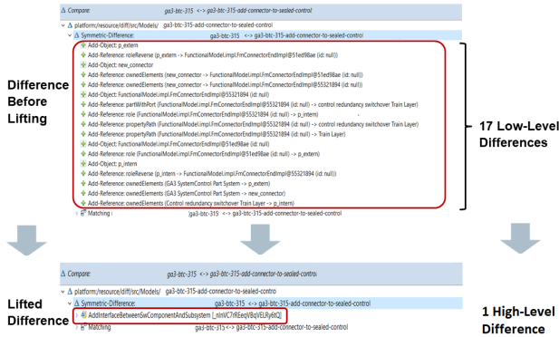
Figure 2: Results of the semantic lifting of a connector that is added between a component and a subsystem.
