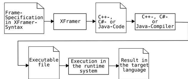
Figure 1. Workflow when applying XFramer [11, p. 57]
