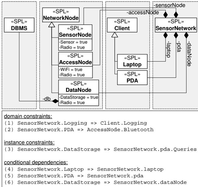
**Figure 5.** A sensor network SPL using network nodes and client applications. The specialized DataNode SPL itself uses a DBMS SPL.
