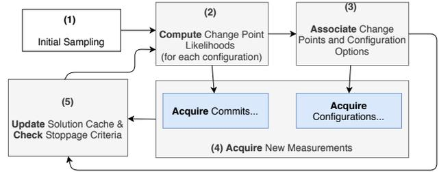
**Figure 3: Overview of our approach:** ① Selecting training data across configuration space and version history, ② estimating the change point probability distribution per configuration, ③ estimating change points as candidate solutions, ④ adaptively augmenting the training set, and ⑤ updating the solution cache and evaluating termination criteria.
