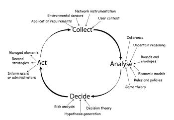
Figure 1. Typical control loop (from [6])
