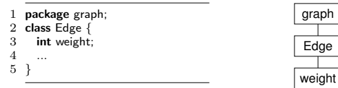
Figure 2: Implementation and FST of feature WEIGHTS (excerpt).
